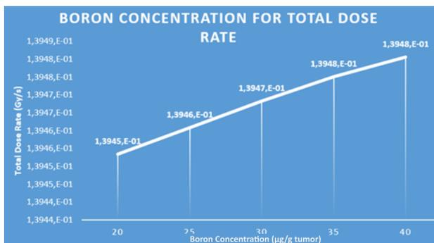
FIGURE 4. Correlation between boron concentration and total absorbed dose rate.
